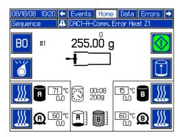
To change the setup of a sequence navigate to Edit Screens #2-#5. See **Screen Navigation Diagram**, page 16.
